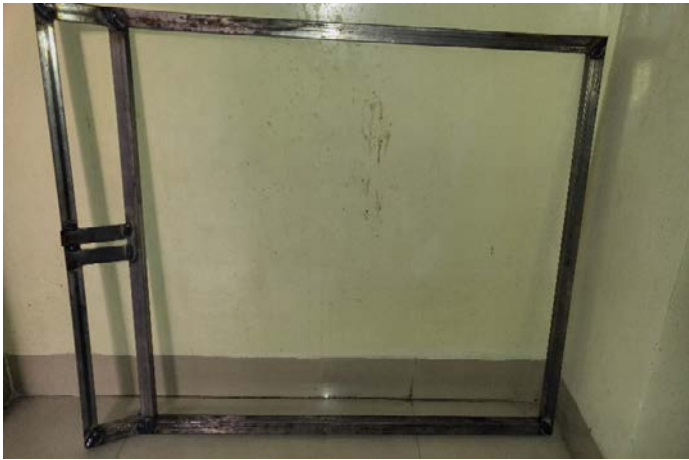
Fig. 7. Fabrication of lower frame
