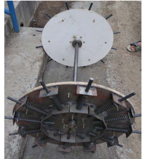
Fig. 5. Fabrication of Blanco wheel and shaft
